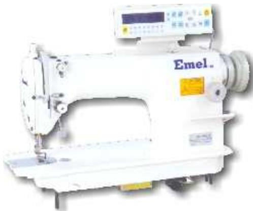
This model is equipped with automatic thread trimmer, automatic needle positioner, automatic thread wipe and many other sewing modes. It is applied to sewing shirt, uniforms and sportswears, and also applied to sewing port folios, purses, shoes, jeans and other medium-heavy weight materials, esp. Suitable for sewing trade marks, pockets, sleeve-cuffs, etc. It can be operated with high quality and high efficiency.
